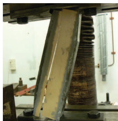
Figure 12: Spruce specimen: Failure of 0% in the glueline.
