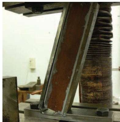
Figure 10: Massaranduba specimen: Failure of 100% in the glueline.
