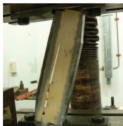
Figure 12: Spruce specimen: Failure of 0% in the glueline.
