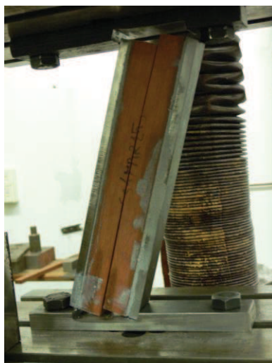
Figure 11: Massaranduba specimen: Failure of 0% in the glueline.
