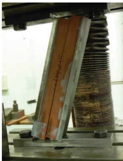
Figure 11: Massaranduba specimen: Failure of 0% in the glueline.
