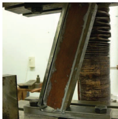
Figure 10: Massaranduba specimen: Failure of 100% in the glueline.
