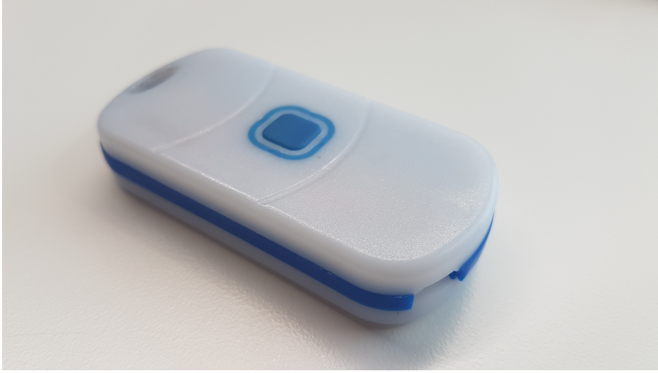
Figure 3.1: One of the mobile LoRa nodes that were carried by volunteers to gather data.
