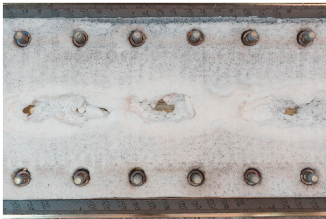
Fig. 14. Distributed insulation damage, photograph taken from the flow side with the liner removed.
