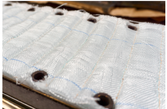
Fig. 10. Example of sample mounting: locally, the liner is mechanically connected to the bottom.
