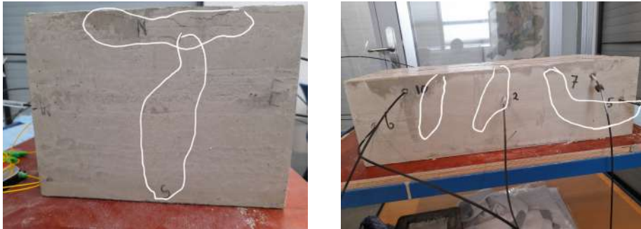
Figure 4.2: Cracks developed after curing
