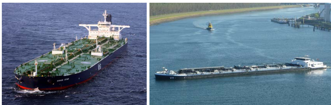
Figure 1.29: Liquid bulk carriers; left: Sea-going ( Sirius Star 2008e by Navy.mil is licenced under CC0 1.0); right: Inland ( Inland tanker vessel by BoH is licenced under CC BY-SA 3.0).
