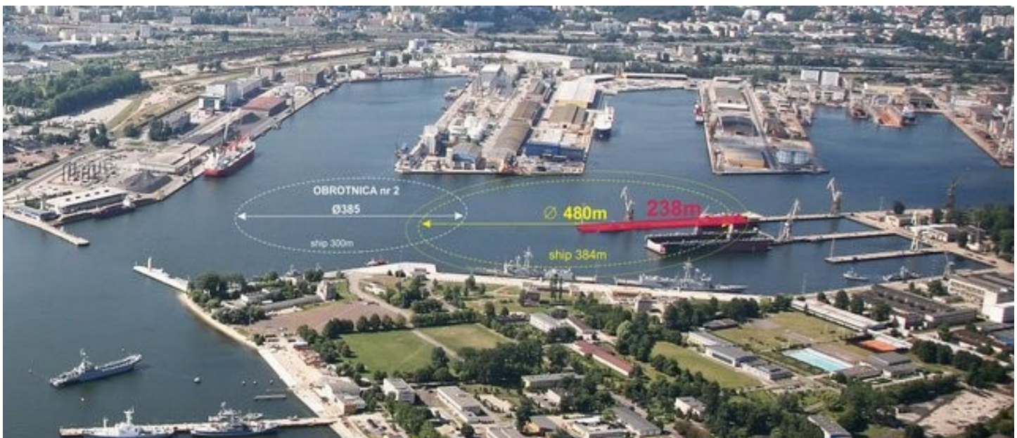
Figure 1.17: Turning basins in the harbour of Gdynia, Poland (Visualization of the concept of redevelopment of the turning basin No. 2 in the port of Gdynia by www.portalmorski.pl is licenced under CC BY 4.0).
