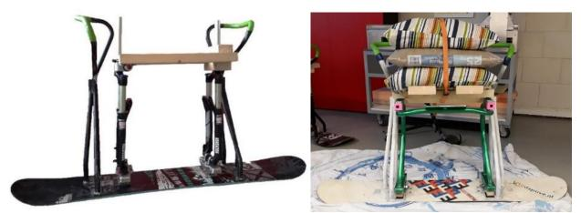
Figure 13: Prototypes for quantitative test. Left: Snowcruiser. Right: Twinrider loaded with dummy weight.
