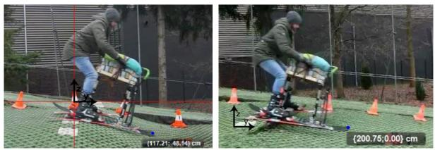
Figure 16: Measurement of contactless distances after hill (left) and sudden drop (right). Screenshots from 'minslow500 run 1'.
