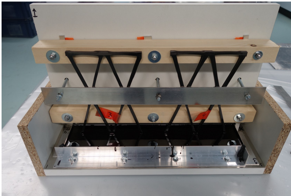
Figure 7.8: Custom mold for casting potting of the test samples.
