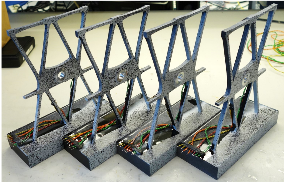
Figure 7.9: Instrumented DC1 samples ready for testing.
