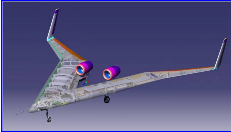
Fig. 5 CAD model of the research vehicle used for inertia estimation
