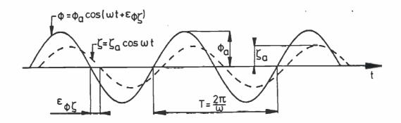
Figure 5.2: Harmonic Wave and Roll Signal
