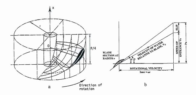
Figure 3.4: Propeller Geometry
