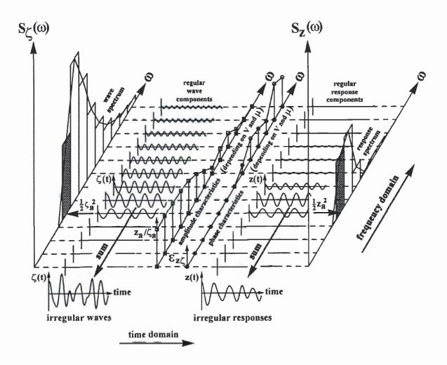
Figure 5.14: Principle of Transfer of Waves into Responses
