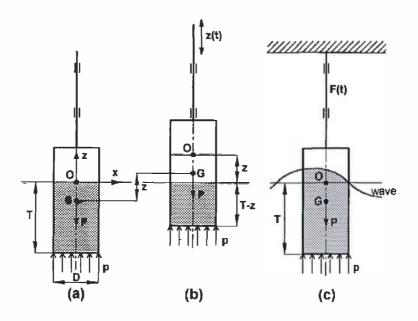
Figure 5.6: Heaving Circular Cylinder
