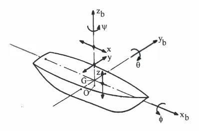
Figure 5.1: Definition of Ship Motions in Six Degrees of Freedom
