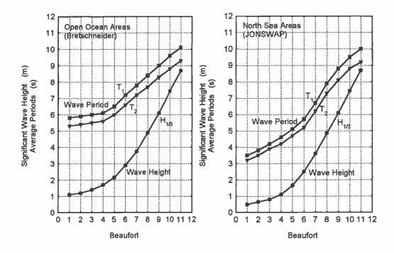
Figure 4.9: Wave Spectrum Parameter Estimates
