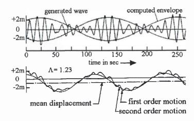
Figure 5.18: Low-Frequency Surge Motions of a Barge
