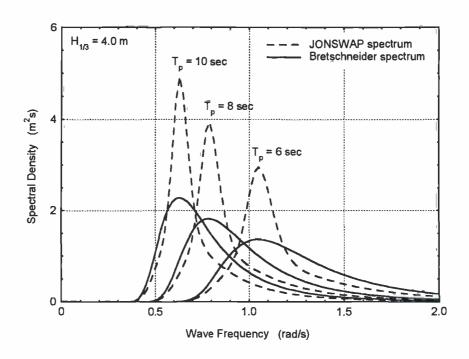
Figure 4.6: Comparison of Two Spectral Formulations
