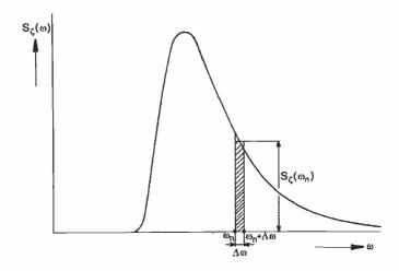
Figure 4.4: Definition of Spectral Density
