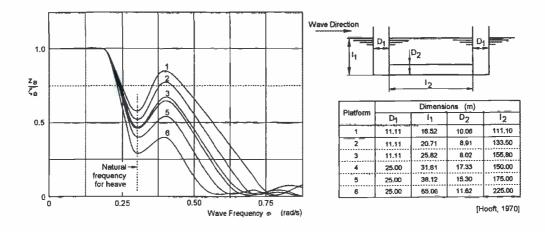
Figure 5.13: Heave Responses of Semi-Submersible Platforms in Waves
