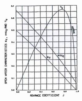
Figure 3.5: Open Water Propeller Diagram
