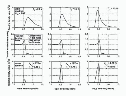
Figure 5.15: Effect of Wave Period on Heave
