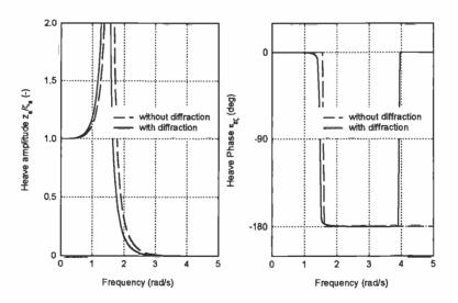
Figure 5.9: Heave Motions of a Vertical Cylinder
