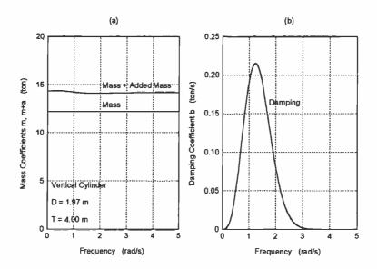
Figure 5.7: Mass and Damping of a Heaving Vertical Cylinder
