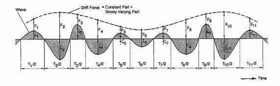
Figure 5.17: Wave Drift Forces Obtained from a Wave Record
