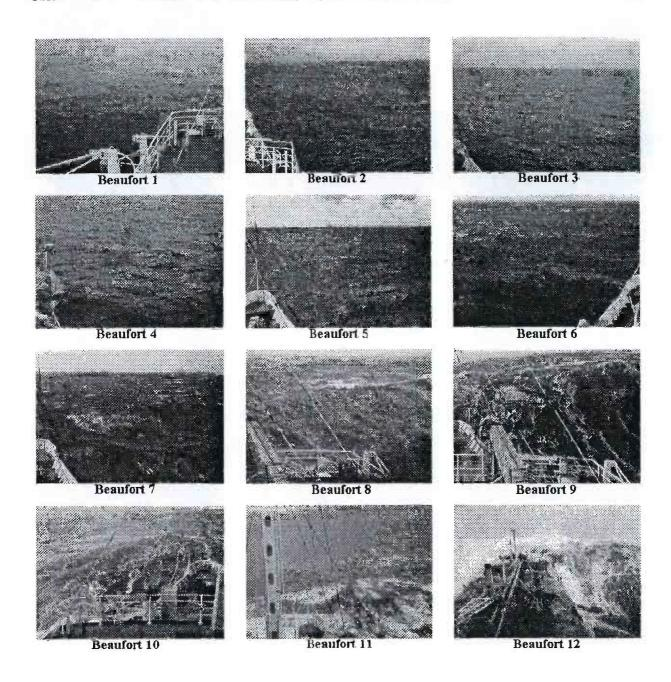
Figure 4.8: Sea State in Relation to Beaufort Wind Force Scale
