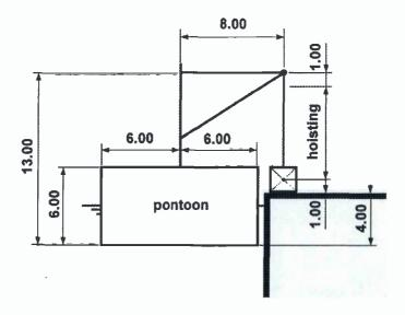
Figure 2.6: Lift Operation by a Pontoon
