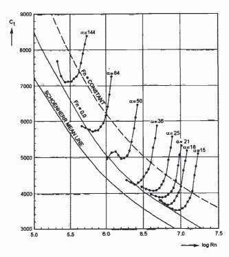
Figure 3.1: Resistance Coefficients of the "Simon Bolivar" Model Family
