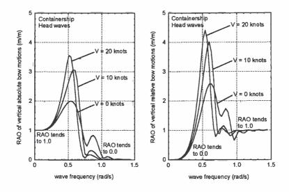
Figure 5.12: Absolute and Relative Vertical Motions at the Bow
