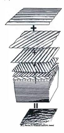
Figure 4.2: A Sum of Many Simple Sine Waves Makes an Irregular Sea
