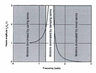
Figure 5.10: Frequency Areas with Respect to Motional Behavior
