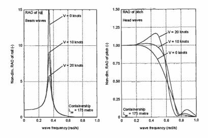
Figure 5.11: RAO's of Roll and Pitch of a Containership
