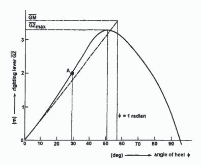
Figure 2.7: Ship Static Stability Curve
