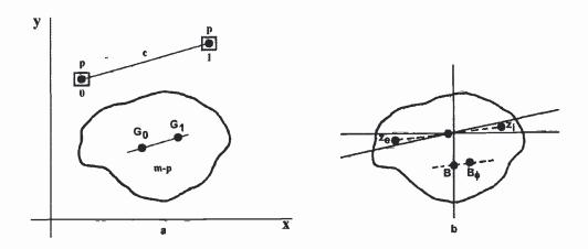
Figure 2.4: Shifting Mass and Buoyancy
