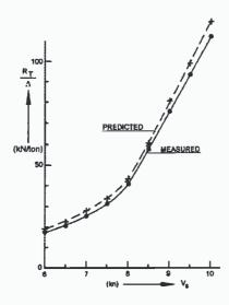
Figure 3.2: Comparison of Resistance Prediction with Model Test Results
