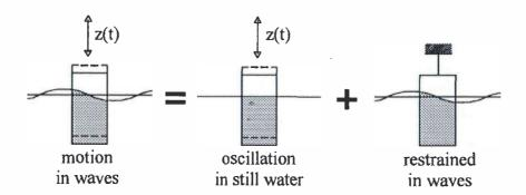
Figure 5.5: Superposition of Hydromechanical and Wave Loads
