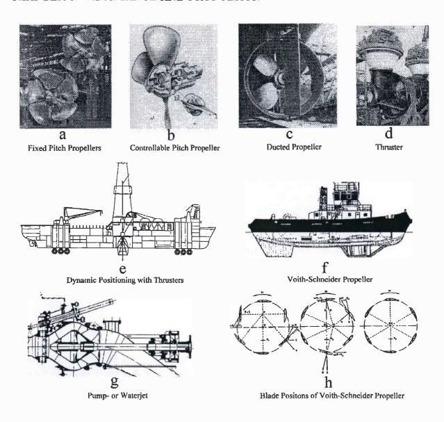
Figure 3.3: Different Propulsion Configurations
