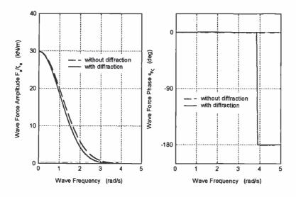
Figure 5.8: Vertical Wave Force on a Vertical Cylinder
