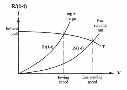
Figure 3.6: Free Running and Towing Speed of a Tug
