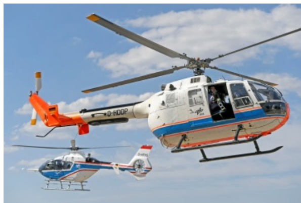
Figure 7.1: Flight experiments with two helicopters for unsteady boundary layer transition measurements on the main rotor of the EC 135, conducted at DLR Braunschweig in June 2018
