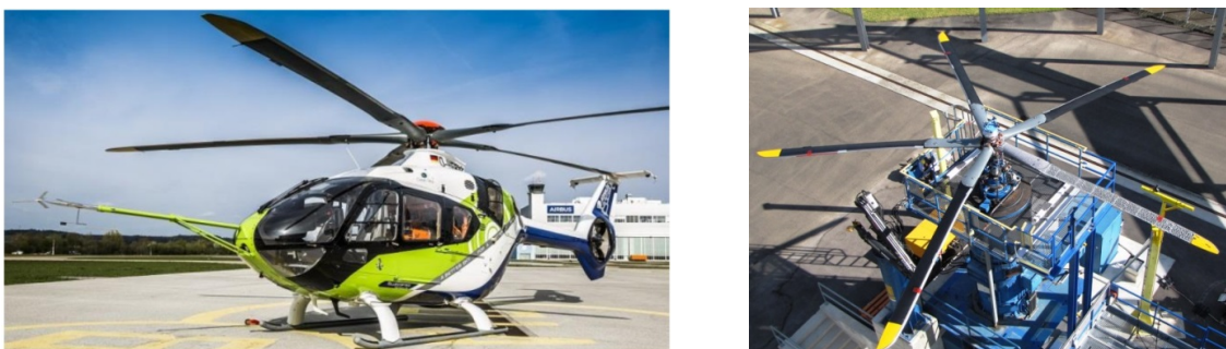
Figure 1.6: GRC1 five-bladed helicopter rotor prototype, from Kus et al. [27]
