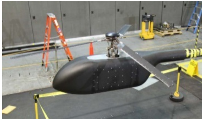
Figure 2.10: Large-scale helicopter model wind tunnel experiment for the application of DIT, from Overmeyer et al. [36]
