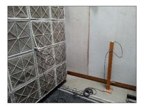
Figure 72: The seventh microphone, which is located some distance away from the inlet.
