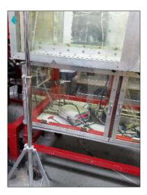
Figure 69: The fourth microphone, which is placed in a separate compartment underneath the test section.
