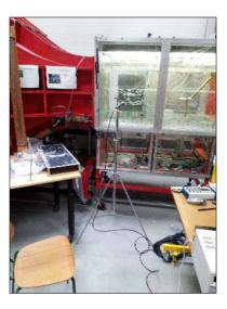
Figure 70: The fifth microphone, which stands next to the test section of the tunnel.
