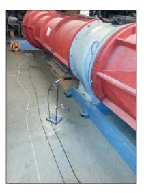
Figure 68: The third microphone, which is placed next to the fan and motor outside of the tunnel.
