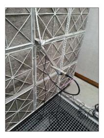
Figure 71: The sixth microphone, which is placed directly in front of the inlet of the tunnel.
