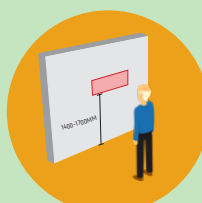
SIGNS ON WALLS ON EYE LEVEL
