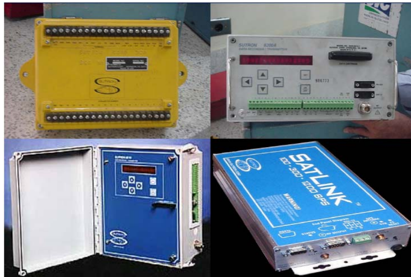
Figure 4.6 SUTRON Data Collection Platforms (DCP's)
