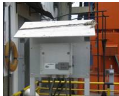
DCP located at the monitoring station at the water intake - Puerto Mallarino Plant
