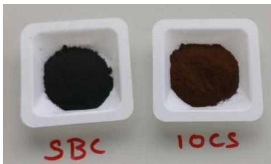
Figure 8 Image showing the sewage-based biochar (left) and iron oxide coated sand (right) used in the research
