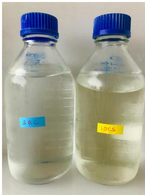
Figure 28 Visual representation of the samples obtained after passing through the columns. Right image: iron-oxide-coated sands effluent, Left image: sewage-based biochar effluent
