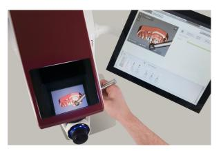
**Figure 1-1:** Simodont training simulator where the procedure of hard tissue removal is practiced with a physical rotary drilling tool.<sup>1</sup>
