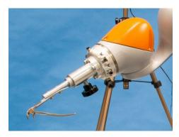
Fig. 4: Holding device for dental forceps.
