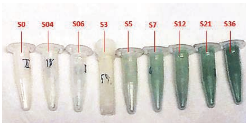
Figure 5.5: Picture of the SrI 2 :Tm 2+ samples in glovesbox. The samples are arranged from low to high Tm 2+ concentration samples and display a clear green colour gradient. The sample names refer to the calculated Tm 2+ concentrations as listed in table 5.5.
