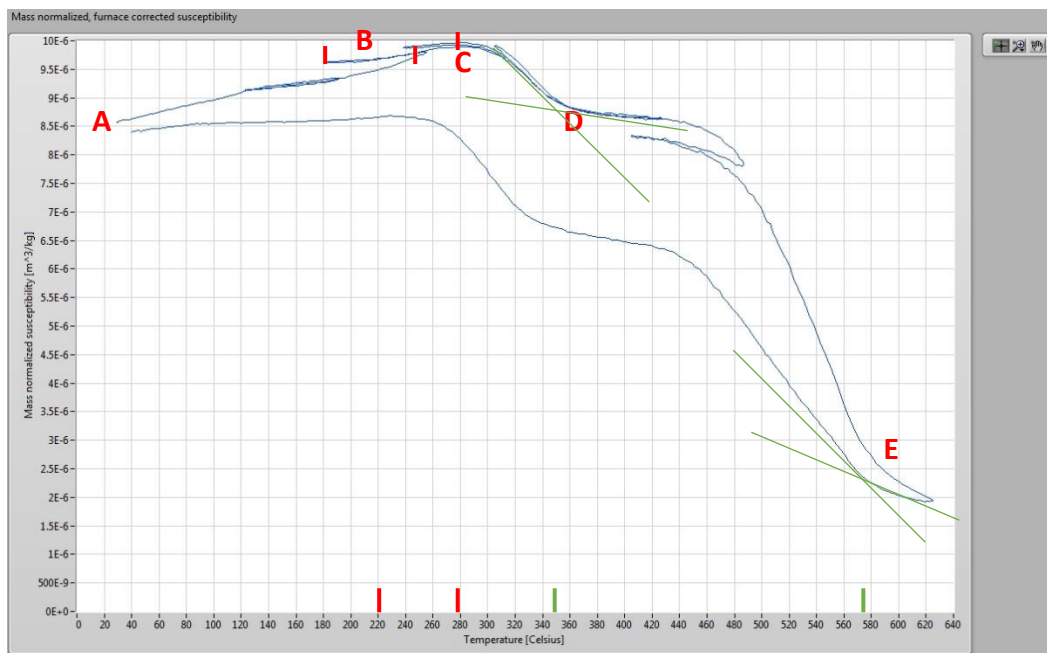
Figure 5 Example of Kappabridge measurements curve. A is the susceptibility at room temperature. B is the point of first alteration (defined by the red stripes) with corresponding temperature (left lower red stripe) and C is the Hopkinson peak (most right upper red stripe) with corresponding temperature (right lower red stripe). Curie temperatures can be obtained from the inflection points after the Hopkinson peak, point D and E, tangent lines in green with corresponding Curie temperatures.
