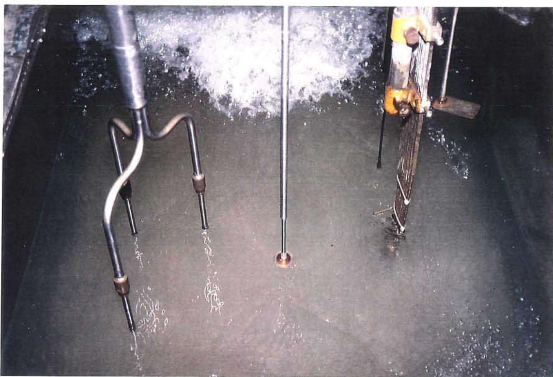
Photo 3.1 The measuring instruments: ASTM, EMS and concentration sampler
