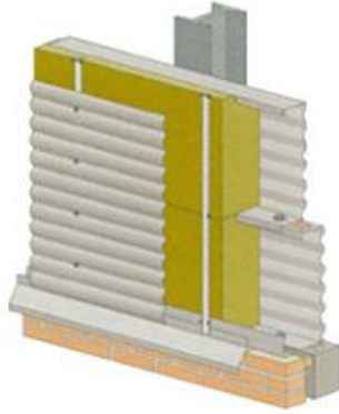
Figure 17: Section of a liner tray system (Architectenweb, 2020)
