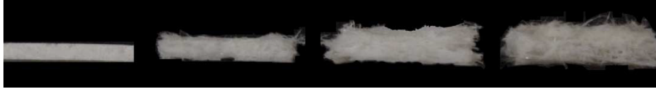
Figure 2.4: Thickness increase due to decompaction in a glass mat thermoplastic (GMT) composite at deconsolidation times: 0s, 50s, 200s and 500s respectively [32]
