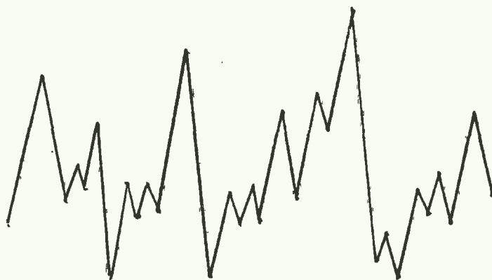
Spectrum after digitizing and conversion of continuous function to straight-line segments joining peaks. Note that even the smallest cycle is retained.
