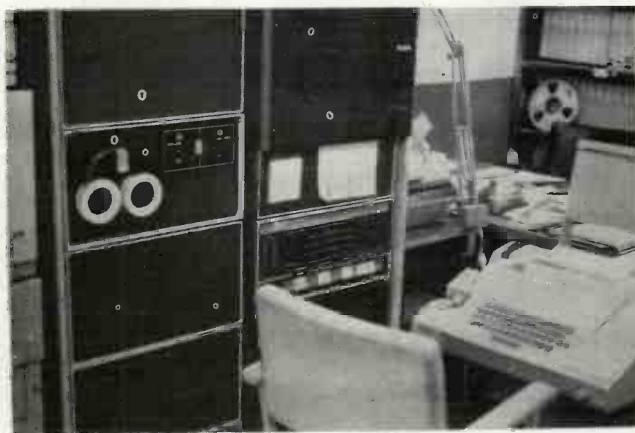
Figure 16. TES PDP-8 Computer for Continuous Monitoring of Random Load Crack Growth
