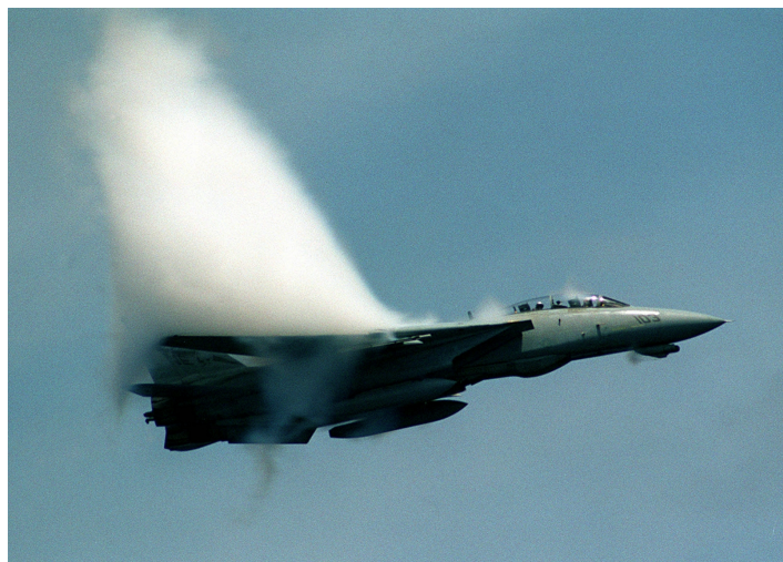
Figure 1.1: F-14D "Super Tomcat" fighter jet flying above critical Mach and experiencing transonic shock waves over the wings
