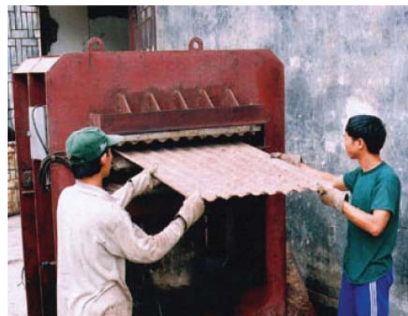
Fig. 4.8: CBRS producing method Source: INBAR, 2006, pp. 1
