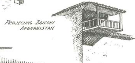
THIS LOGGIA IS PARTLY WINDOWED, PARTLY OPEN, AND PARTLY FITTED WITH LOUVERED SHUTTERS.
