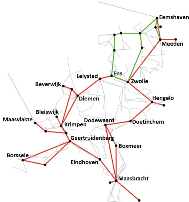
Figure 8.3: Representation of the Dutch transmission network, based on the model’s input dataset. 380kV and 220kV (EHV) lines are colored in red and green, respectively. 150kV and 110kV (HV) lines are colored in gray. Major substations are labeled for reference.
