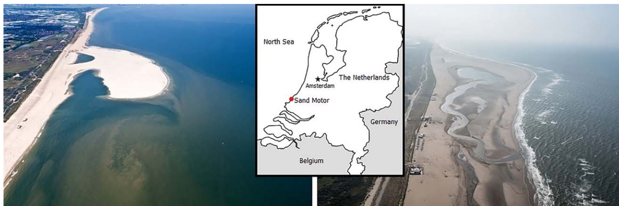
Figure 1. The Sand Motor mega-nourishment in the Netherlands (left) just after construction in 2011, with turbidity patterns at the sea surface revealing signs of a separating tidal flow field, and (right) in 2014, after approximately 3 years of morphological development. Images by Joop van Houdt/Rijkswaterstaat.
