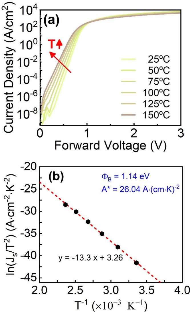
**Figure 5.** (a) Forward  $J$ - $V$  characteristics of quasi-vertical GaN SBD with post-mesa nitridation in semi-log scale at temperatures ranging from 25 °C to 150 °C and (b) corresponding Richardson plot.
