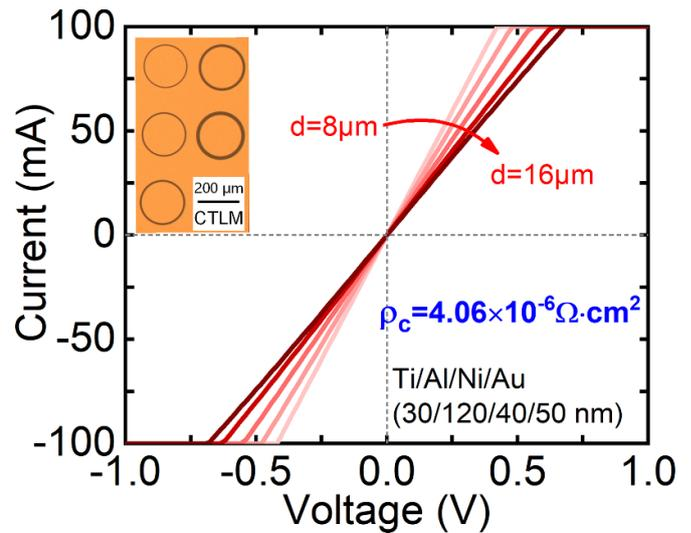
**Figure 2.** The  $I$ - $V$  curves of Ti/Al/Ni/Au contact on  $n^+$ -GaN as a function of contact spacing, measured from CTLM patterns. The inset is an optical microscopy image of CTLM patterns. The inner radius of the measured pattern was 100  $\mu\text{m}$  with a different spacing of  $d$  ( $d = 8, 10, 12, 14, 16 \mu\text{m}$ ) to the outer ring.
