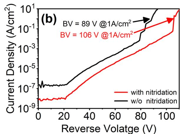
**Figure 3.** (a) Measured forward  $J$ - $V$  (left) and  $R_{\text{ON,sp}}$  (right), and (b) reverse  $J$ - $V$  characteristics of the quasi-vertical GaN SBD with post-mesa nitridation and the reference with an anode diameter of 70  $\mu\text{m}$ .
