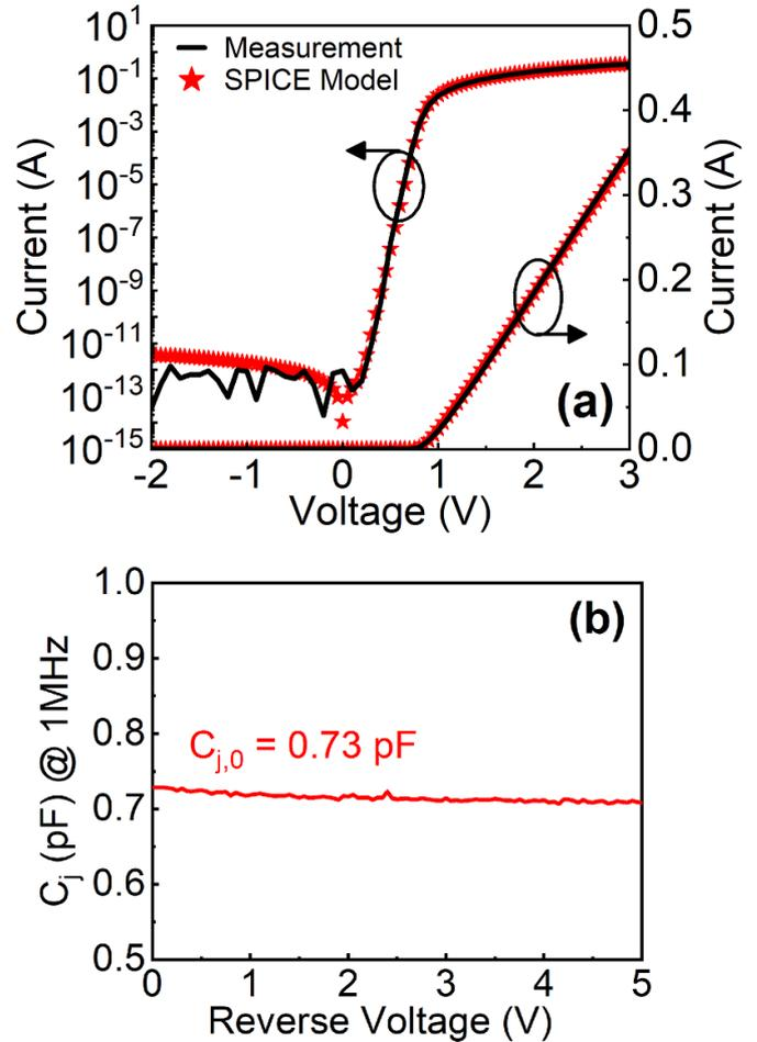
**Figure 6.** (a) Measured and simulated forward  $I$ - $V$  in semi-log scale and in linear scale (right). (b)  $C$ - $V$  characteristics of quasi-vertical GaN SBD with post-mesa nitridation with an anode diameter of 70  $\mu\text{m}$ .
