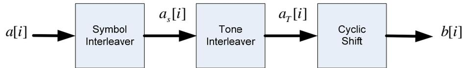
**Figure3.7** Block diagram of three stage bit interleaver [2]
