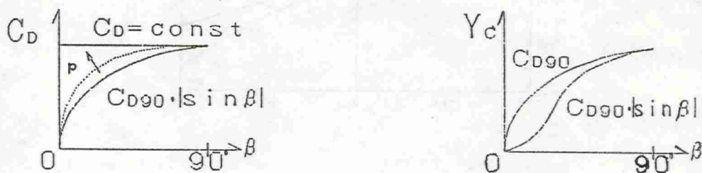
Fig. 7 Cross-flow drag coefficient and its effects at r=0
