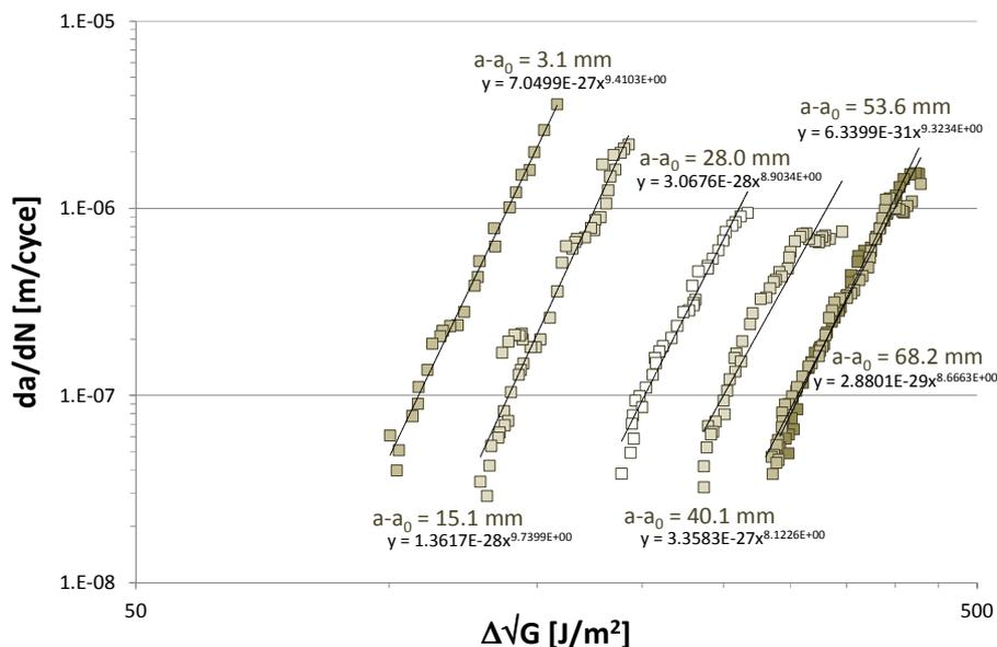
**Figure 1.** Six successive delamination resistance curves obtained from a single specimen, labelled specimen 7 in [26]
