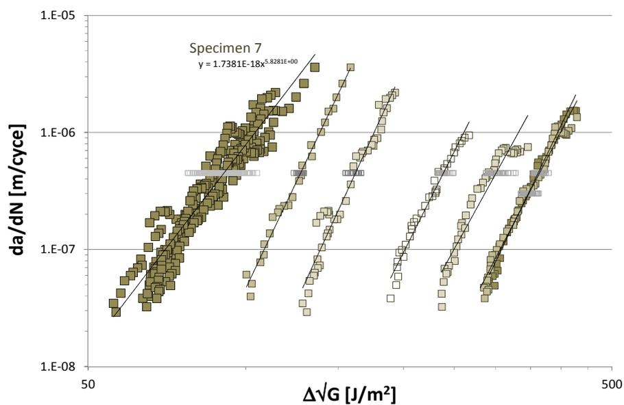
Figure 5. Comparison between the translated curve and the original six curves from specimen 7 in [26]
