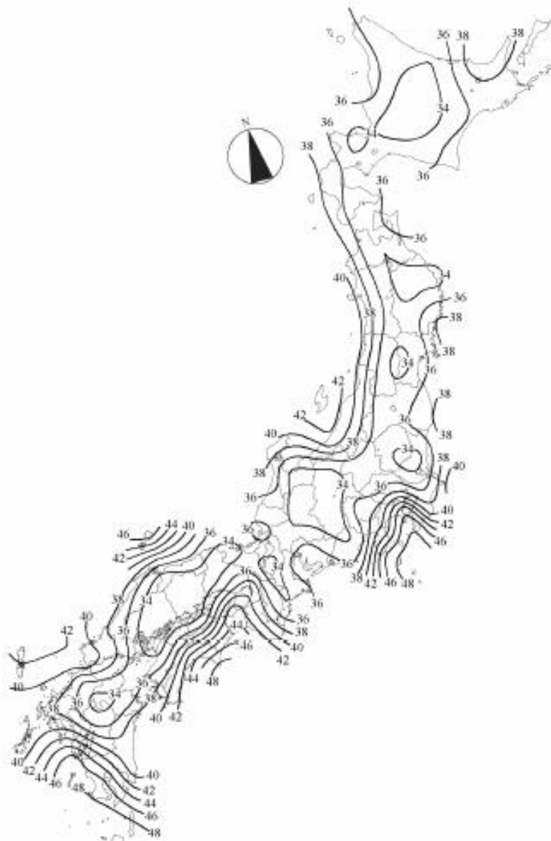
Figure 2.21: Basic wind speed Japan, U_{500} [Tamura, Y., Kawai, H., Uematsu, Y., Okada, H., Ohkuma, T., 2004]
