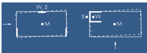
Figure 3.20: Asymmetric bracing [Bachmann, H, 2003]
