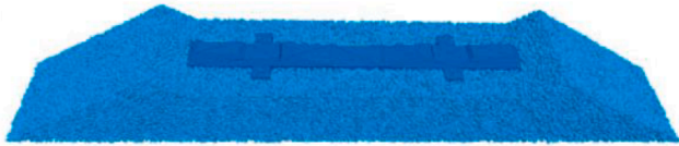
Fig. 2. DEM model of a single sleeper (wing-shape) section [8].
