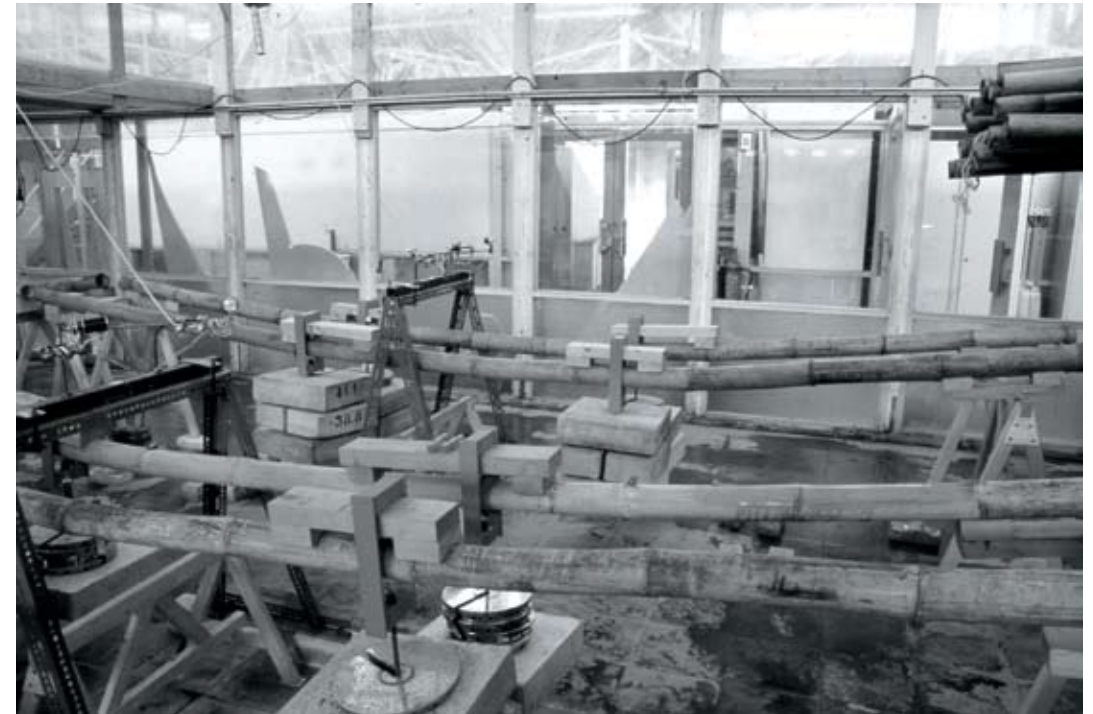
Fig. E1: Bending test, performed at the Technical University of Eindhoven (1981-1988).
