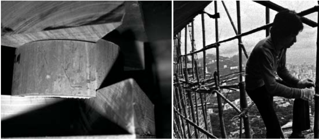
Fig. E.3: A test on shear, performed in Costa Rica, according to a test method developed at the Technical University of Eindhoven in the 1970s. Fig. E.4: A man working at a bamboo scaffolding of a high rise building in China (National Geographic, 1987)
