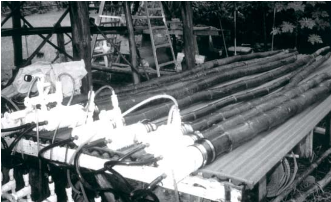
Fig. 6.4: Bamboo poles being treated with the Boucherie preservation technique
