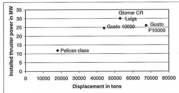
installed power per ton displacement, see figure below.
