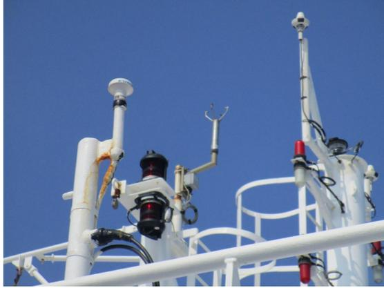
Figure 1.7: Windsensor on top of the wheelhouse - Happy star
