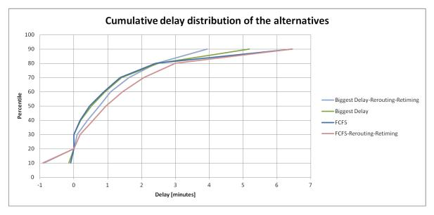
Figure 5.4: Cumulative delay distributions for the alternatives consisting of reordering, rerouting and retiming combined with the distributions of the two 'best' prioritisation algorithms.
