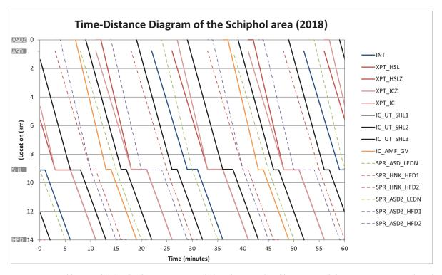
Figure 4.5: Possible timetable for the future situation including the XPT. The abbreviations of the train series are explained below in table 4.2. The timetable is showed in the form of a time distance diagram where the branch from Amsterdam Zuid and Amsterdam Lelylaan are plotted on top of each other.
