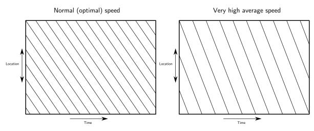
Figure 2.9: Left a low speed train service with relatively small buffers needed for a stable service. On the right a high speed train service where relatively large buffers are needed for a stable service.
