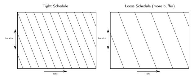
Figure 2.8: Left a tight schedule with limited buffer times included, which is less stable during disruptions. On the right a more 'loose' schedule with lots of buffer times, which are very usable for recovery of disrupted situations.
