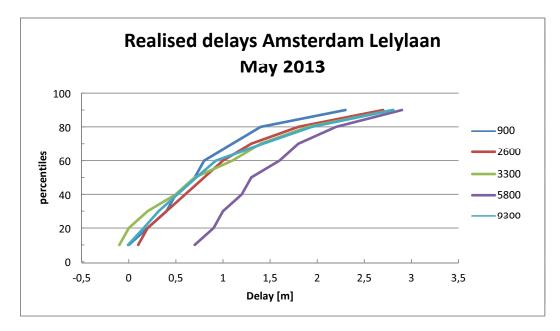
Figure 4.13: Realised delays of train series coming from the direction of Amsterdam Lelylaan (Amsterdam CS etc.) and heading for Schiphol and further.
