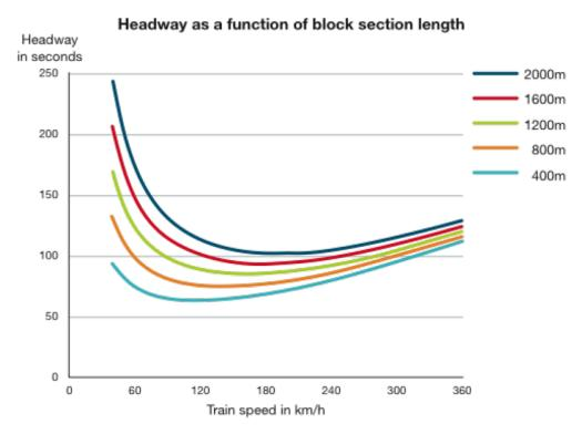
Figure 2.6: The minimum headway as function of the maximum speed and the block length using ERTMS level 2 (Hunyadi, 2011).
