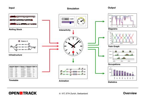
Figure 4.1: Overview of the functionalities of OpenTrack with the required input and the produced output (Huerlimann, 2013).
