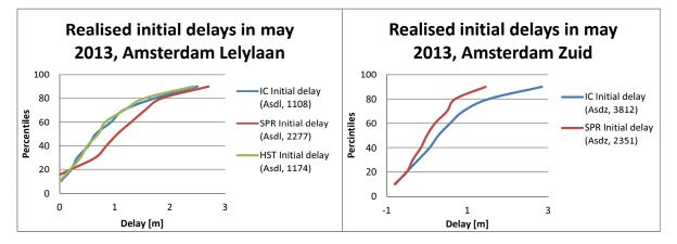
Figure 4.6: Realised initial delays in may 2013 measured at Amsterdam Lelylaan and Amsterdam Zuid. Displayed per train type, including the total amount of trains measured. (Data from ProRail and NS)
