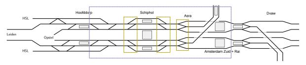
Figure 2: Overview of the 2018 Schiphol railway network. The large, blue area shows the control area of the DVM system. The smaller, orange areas show the steering areas.
