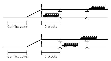
Figure 4.7: The double threshold system for prioritisation. The first situation does not require prioritisation, the second one does.
