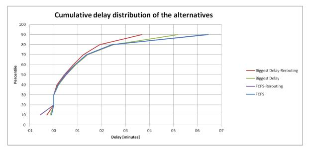
Figure 5.2: Cumulative delay distributions for the alternatives consisting of reordering and rerouting combined with the distributions of the two 'best' prioritisation algorithms.
