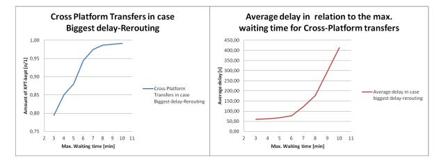
Figure 5.6: Showing the relation between the amount of XPT-connections kept and the XPT maximum waiting time (left) and the relation between the average delay caused in the system and the XPT maximum waiting time.
