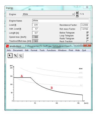
Figure 4.4: Example of what the rolling stock data looks like in OpenTrack, with the entry fields of the basic data and the traction-force curve. A is the traction-force limited due to adhesion, and B is limited by the engine power. (OpenTrack).
