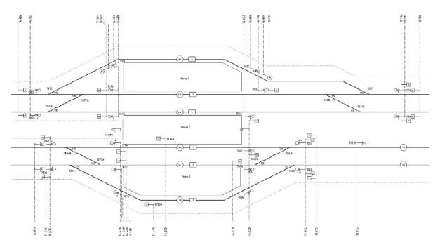
Figure 4.3: Example of a part of an OBE-sheet, of Schiphol (NS / ProRail).
