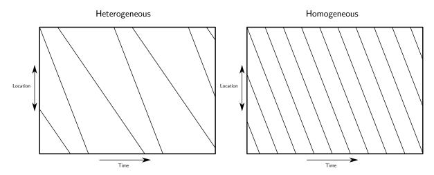
Figure 2.7: Left a heterogeneous utilisation of a track as seen in a classical two train (local and express) service pattern. On the right a homogeneous utilisation of a track which results in a much higher amount of trains per hour but will not satisfy all the customers their demands.
