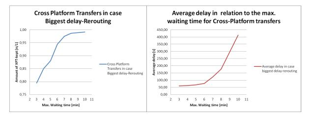
Figure 3: Showing the relation between the amount of XPT-connections kept and the XPT maximum waiting time (left), and the relation between the average delay caused in the system and the XPT maximum waiting time.
