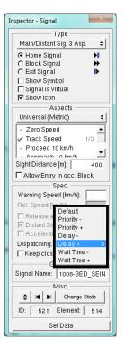
Figure 4.8: The settings of a signal in OpenTrack where prioritisation can be determined for the route setting in case of a conflict.
