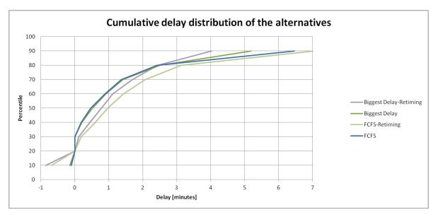
Figure 5.3: Cumulative delay distributions for the alternatives consisting of reordering and retiming combined with the distributions of the two 'best' prioritisation algorithms.
