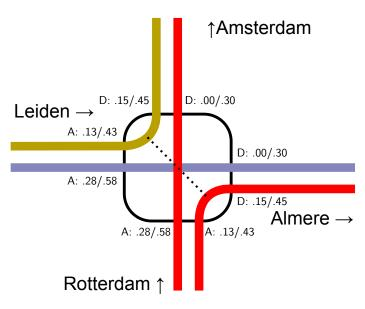
Figure 3.5: Concept of the alternating IC/HST services at Schiphol with a frquency of two times per hour per line. The dotted line shows the transfer relations. The times are only indications, a shift in time in the schedule is always possible.
