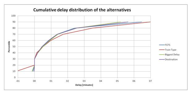
Figure 5.1: Cumulative delay distributions for the four prioritisations tested in OpenTrack.
