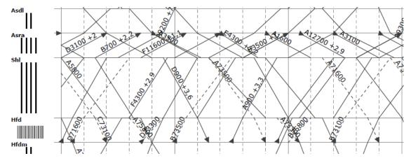
Figure 2.3: Time distance diagram of the Schiphol area with a 'width' of 30 minutes (ProRail).
