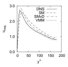
Figure 4: RMS of velocity fluctuation in the streamwise direction
