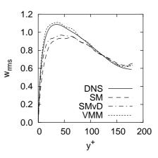
Figure 6: RMS of velocity fluctuation in the spanwise direction
