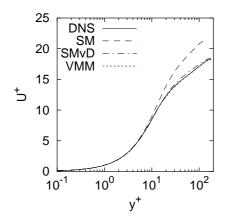
Figure 3: Mean streamwise velocity
