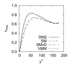
Figure 5: RMS of velocity fluctuation in the wall-normal direction
