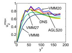
Figure 9: RMS of velocity fluctuation in wallnormal direction
