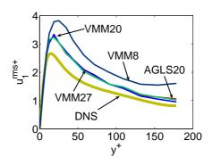
Figure 8: RMS of velocity fluctuation in streamwise direction
