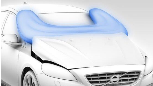
Volvo pop-up bonnet with pedestrian airbag
