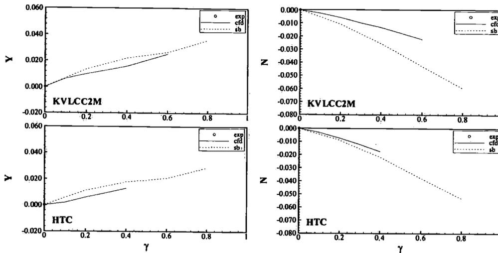
Figure 6: Comparison between predicted forces for yaw rotation using viscous flow calculations and using slender-body method
