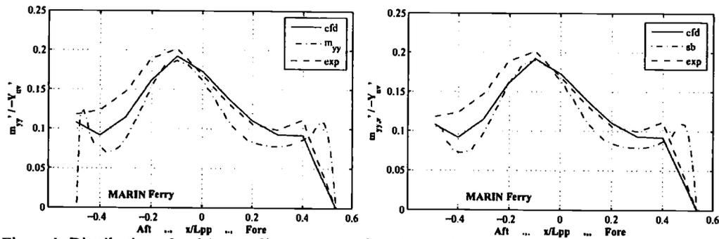
Figure 1: Distribution of real ( $m_{yy}$ , left) and virtual (sb, right) sectional transverse added mass
