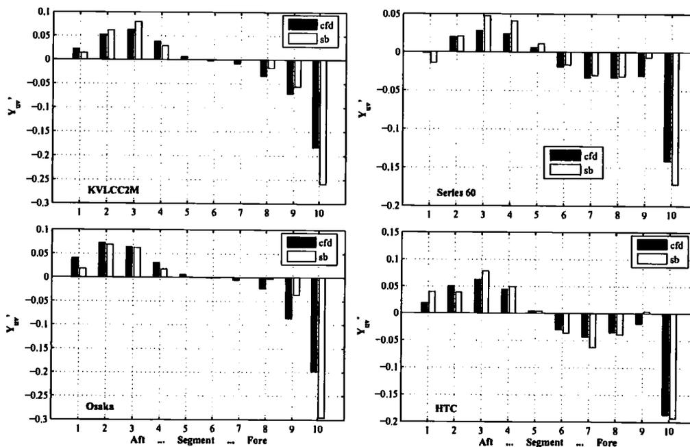
Figure 3: Distribution of sway force derivative for drift along the segments
