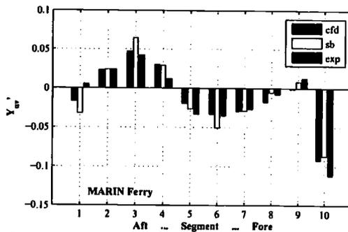
Figure 2: Distribution of sway force derivative for drift along the segments (MARIN Ferry)
