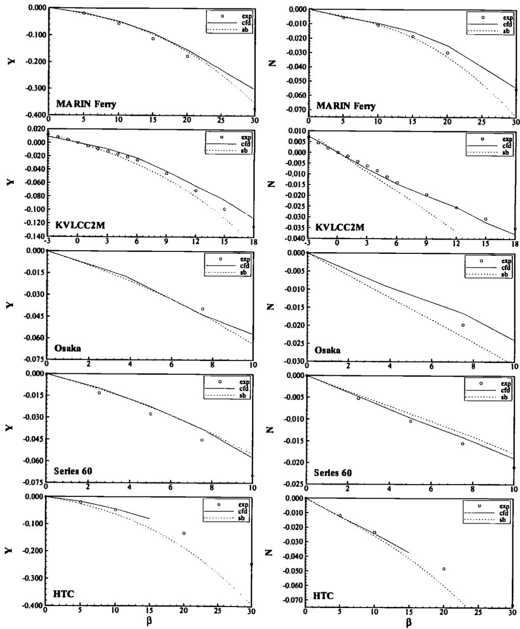
Figure 5: Comparison between predicted forces for drift using viscous flow calculations and using slender-body method
