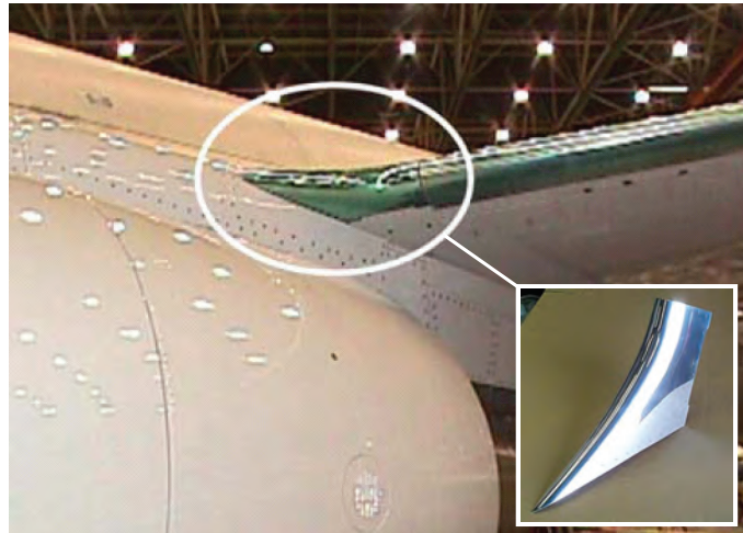
Figure 3.5 – SPF AA5083 strakelet on the 737 wing leading edge (adapted from [98])
