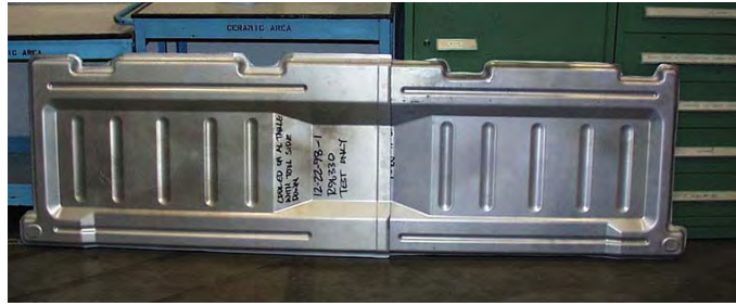
Figure 3.4 – 767 superplastically formed moisture shroud assembly comprised of two SPF AA5083 components [98]
