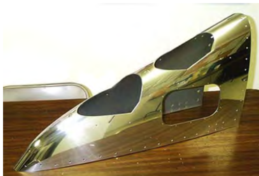
Figure 3.3 – SPF AA5083 777 wing tip light housing [98]
