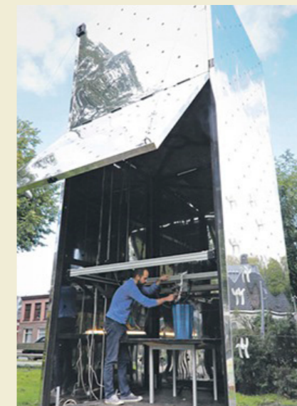
Figure 2.7: KamerMaker 3D Printer (Honka, 2013)
