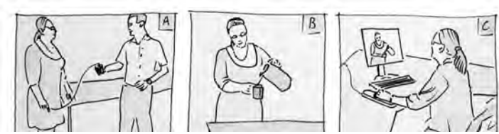
Figure 4.1. Approach to the measurement of the dynamics of emotion in person-product interaction 2 A: Physiological recording equipment can be attached for ambulatory measurement during the test. B: The test participant interacts with the product freely while being filmed. C: Video of the product test is presented immediately to collect emotion ratings
