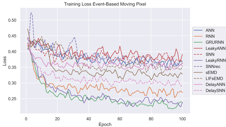
Figure 6.2: Training loss for the event-based 1D moving pixel task. For better readability the running average of the loss of two subsequent epochs are plotted.
