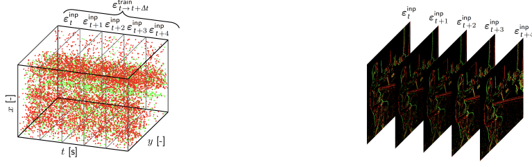
Fig. 2: Left: Schematic representation of the output event stream of the event camera. Discrete partitions in the time dimension are created every \Delta t seconds. Right: The resulting frames after the events within each partition are accumulated. Images are a courtesy of [23].
