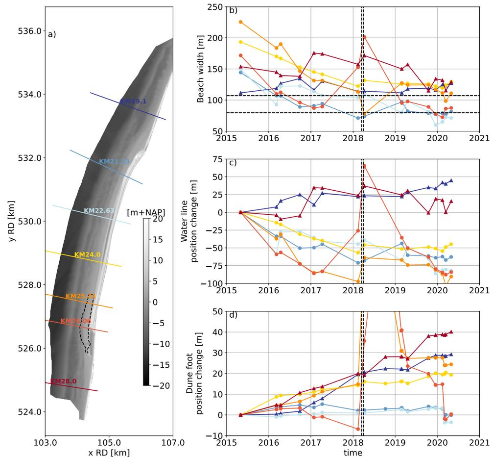
**Figure 12.** Beach width in time for transects 19.1, 21.23, 22.63, 24, 25.31, 26.06, and 28. (a) Location of transects. (b) Beach width. (c) Waterline position change. (d) Dune foot position change. The black dotted horizontal lines indicate the  $\mu \pm \sigma$  beach width at the adjacent coast. The black dotted vertical lines indicate the period of the additional 2018 beach nourishment. Eroding and accretive transects are marked with circle and triangle symbols, respectively.
