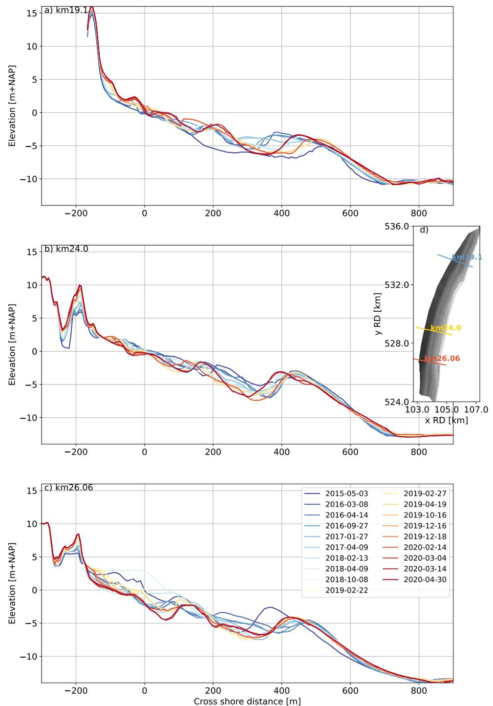
**Figure 6.** Bed levels on three cross-shore transects. (a) Northern transect at km 19.1. (b) Central transect at km 24.0. (c) Southern transect at km 26.06. Colors show the different surveys in time. (d) the location of the transects in plan view. 0 m + NAP is approximately MSL.
