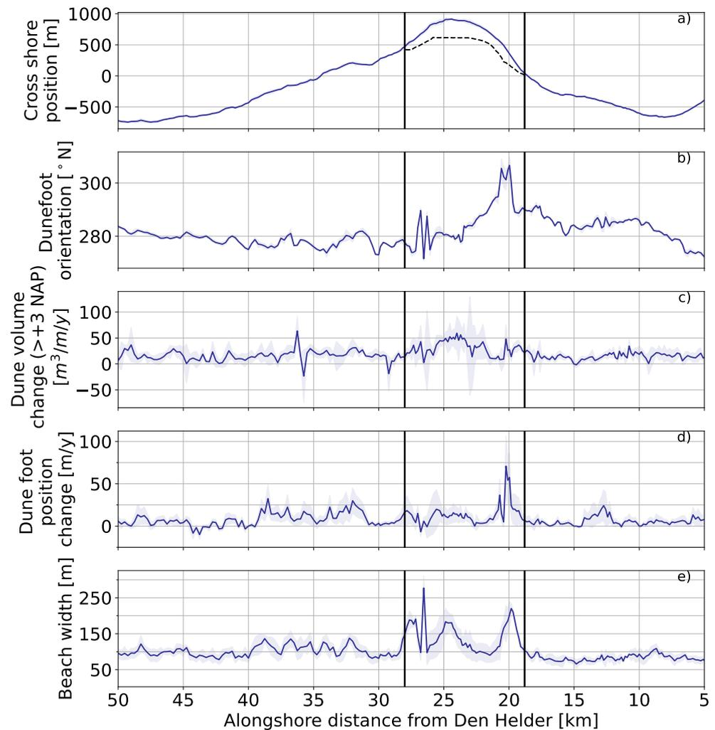
**Figure 11.** Dune evolution of North-Holland coast with the nourished section in between black lines (JARKUS dataset only). (a) Cross-shore position of the waterline (relative to the waterline position at km 0.2); the position of the prenourishment waterline is in black stripes. (b) Orientation of the dune foot. (c) Dune volume change, above 3 m + NAP. (d) Dune foot position change. (e) Beach width.
