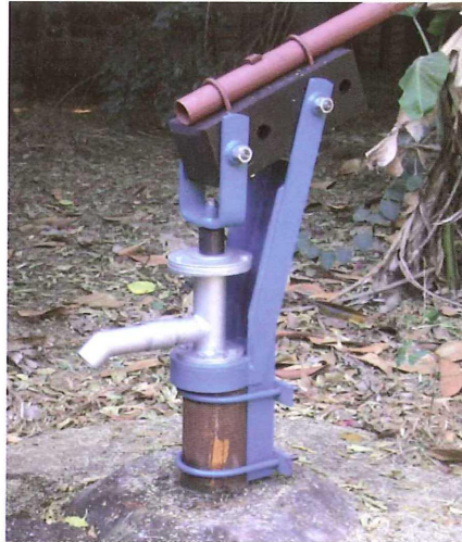
Fig 19. The Zimbabwe Bush Pump {Source: Morgan, P. 2009}
