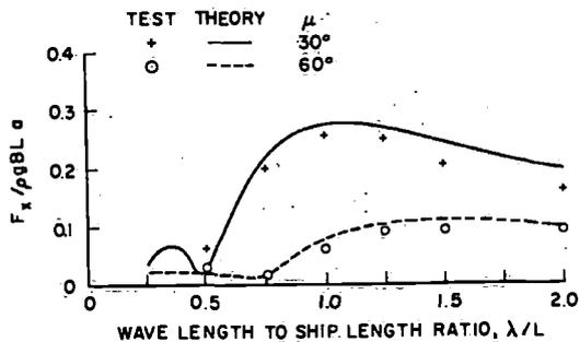
FIG. 9. AMPLITUDE OF SWAY-EXCITING FORCE FOR SERIES 60 MODEL
