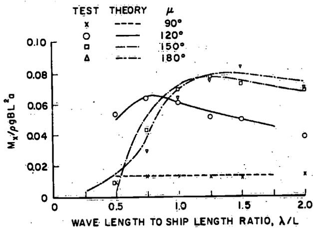
FIG. 17. AMPLITUDE OF PITCH-EXCITING MOMENT FOR SERIES 60 MODEL
