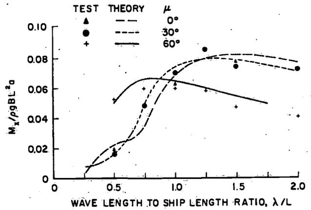
FIG. 16. AMPLITUDE OF PITCH-EXCITING MOMENT FOR SERIES 60 MODEL
