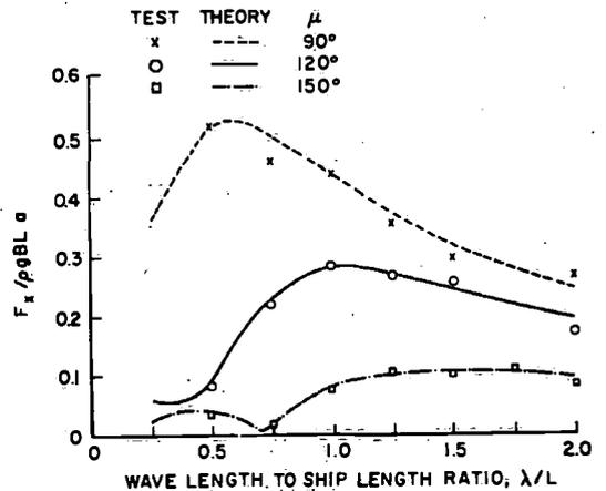
FIG. 10. AMPLITUDE OF SWAY-EXCITING FORCE FOR SERIES 60 MODEL
