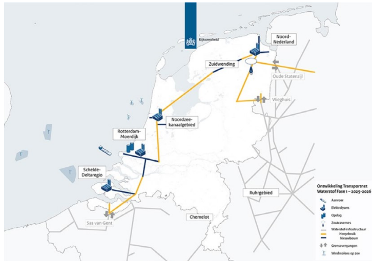
Figure 12: First phase of Hydrogen Backbone.
