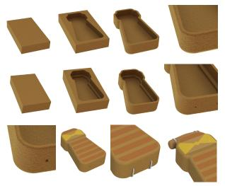
Figure 4.26: production steps: 1. bottom block 2. milling inside 3. milling outside 4. sanding 5. top block 6. milling inside 7. milling outside 8. drilling holes 9. sanding 10. paiting 11. attach cord 12. attach handle
