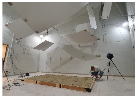
Figure 5 - Reverberation room measurements
