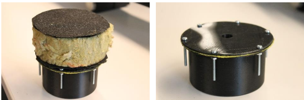
Figure 37 - Used samples. (A) multilayer setup, (B) the resonator with inward neck
