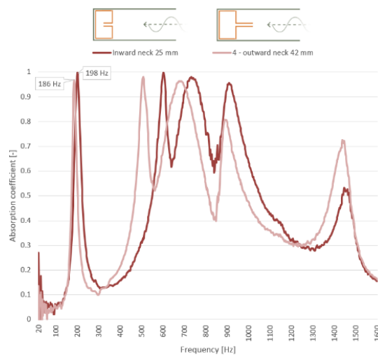
Figure 30 - Control tests for resonators with neck
