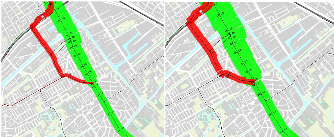
Fig. 3: Relative network effects [% ridership change] of frequency increase on link loads a) without considering comfort (left) and b) considering comfort effects (right) during a morning peak.
