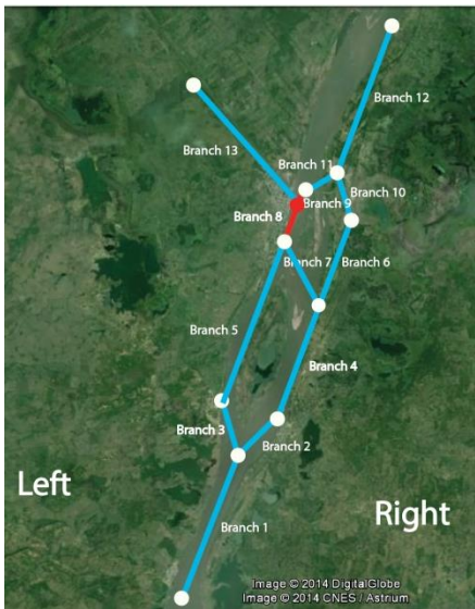
Figure C. 6- Schematisation bifurcation with changed position of the offtake (marked red)
