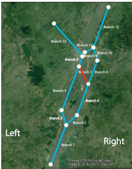
Figure C. 17- Schematisation bifurcation width mid channel (Branch 7) marked in red
