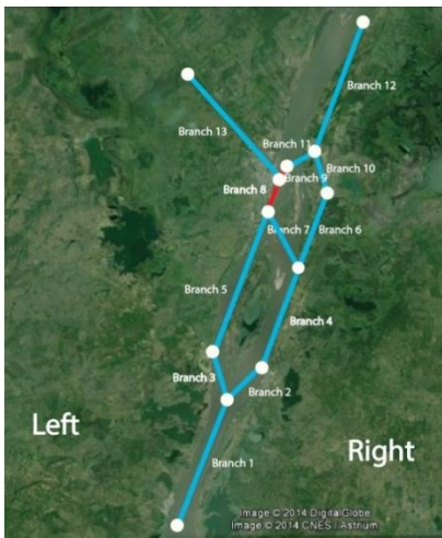
Figure C. 19 - Schematisation bifurcation width branch 8 and 9 marked in red
